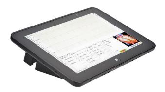
The InterSim® III Touch is used to simulate the human heart. In combination with the InterSim® III Adapter Box, the electrical and electrochemical properties of the cardiac system of humans can be simulated and the interaction with implantable pacemakers and defibrillators can be learned.
